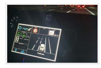
Emergency vehicle approaching Traffic Jam Ahead Warning **GLOSA/SPAT** Road Works Warning **Smart Routing**
